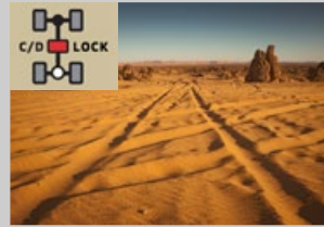
4HLC (4WD High Range with locked centre differential) For low-grip surfaces like unsealed roads and sand.
